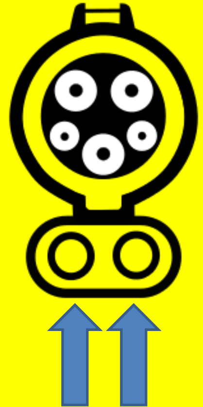
High Voltage DC Connections
